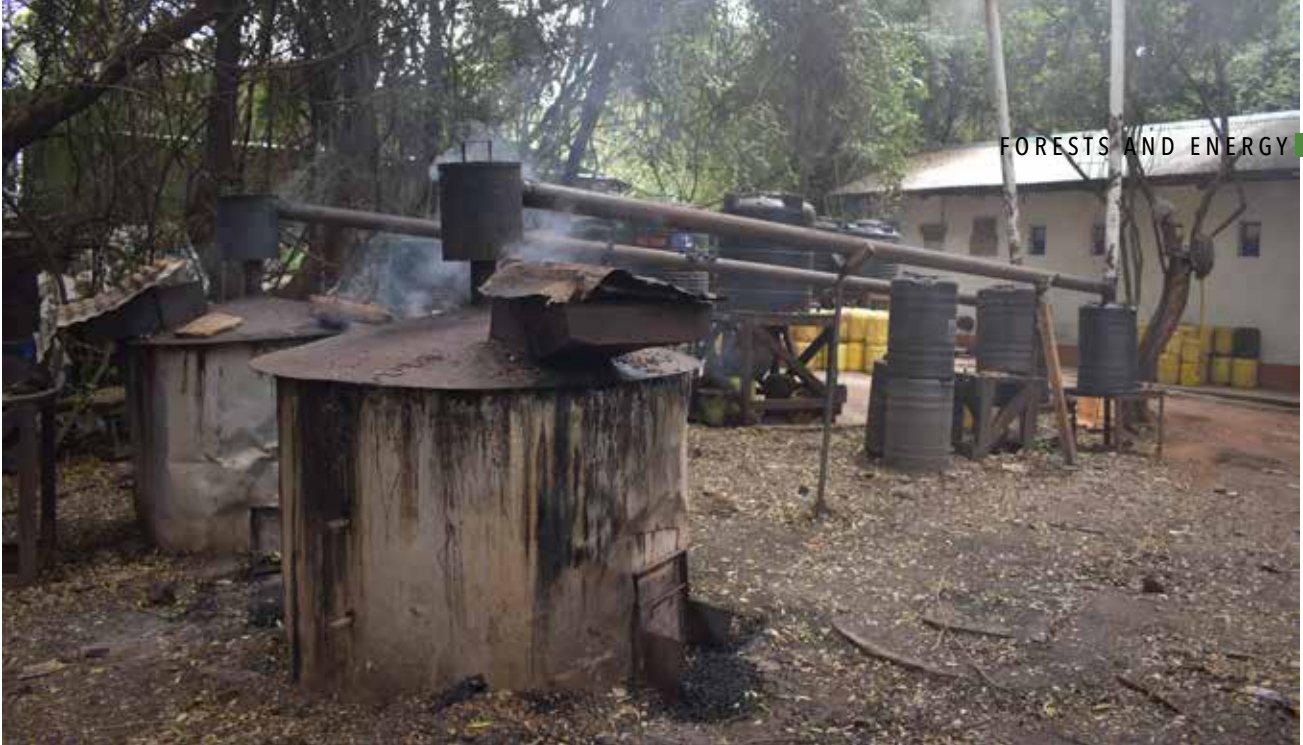
The pyrolysis equipment, in operation
