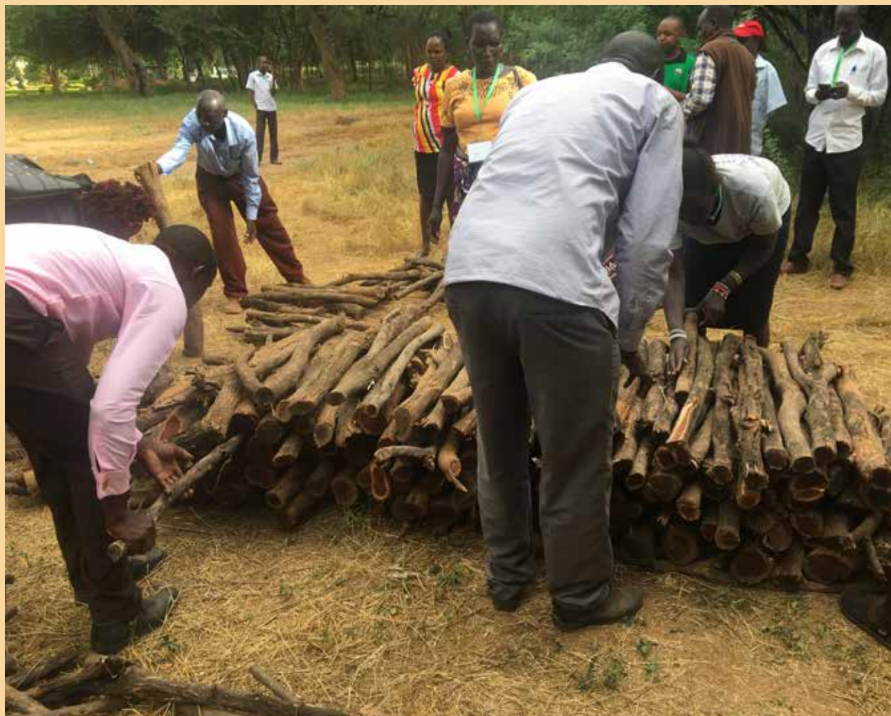
Stacking wood tightly to reduce air spaces and enhance heat transfer. Photo Mary Njenga/ICRAF
