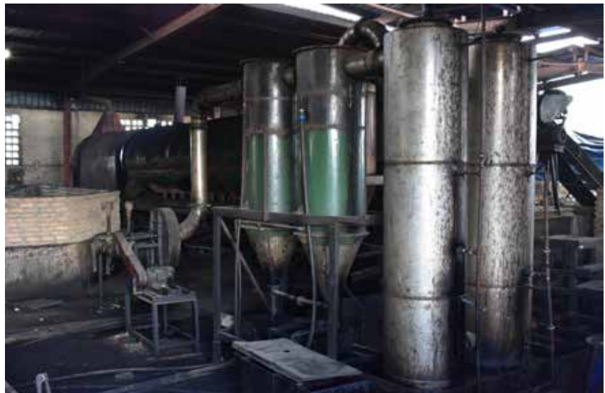
The furnace, with cyclones (greenish) and cleaning cylinders, and the pump through which the syngas is fed to the burners (at the bottom of the furnace).
